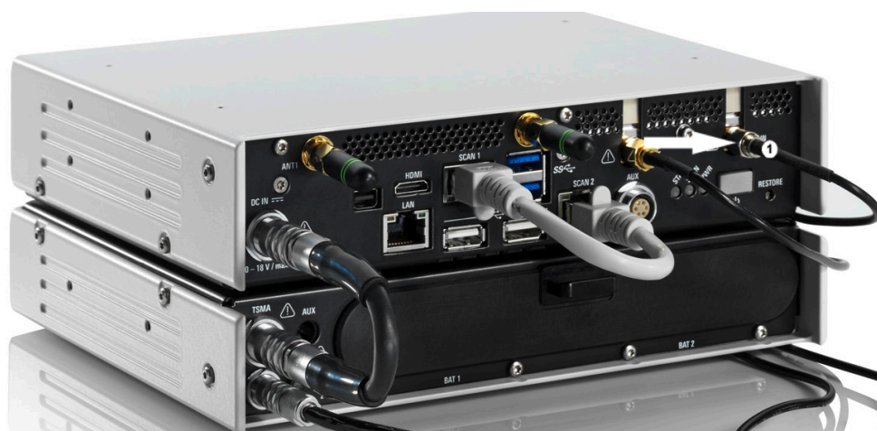
Figure 5-8: R&S TSMA Antenna Cabling - RF
