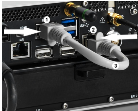
Figure 5-5: Connection between scanner unit and internal PC unit
