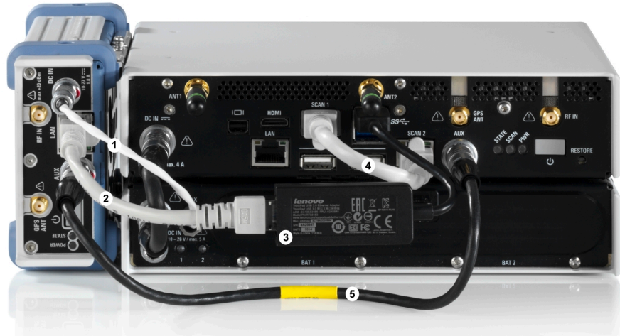
Figure 2-19: Cabling of R&S TSME with R&S TSMA
