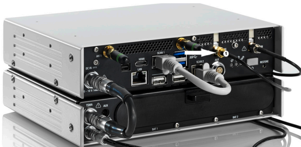
Figure 5-7: R&S TSMA Antenna Cabling - GPS
