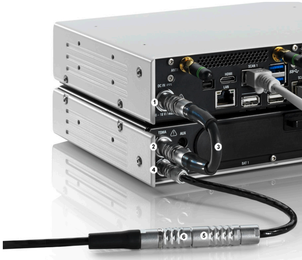
Figure 2-13: Connecting the R&S TSMA with an AC power supply
